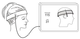
Figure 1. Personalized tourniquet system, with cuff applied to patient scalp and instrument displaying applied cuff pressure and inflation time.
