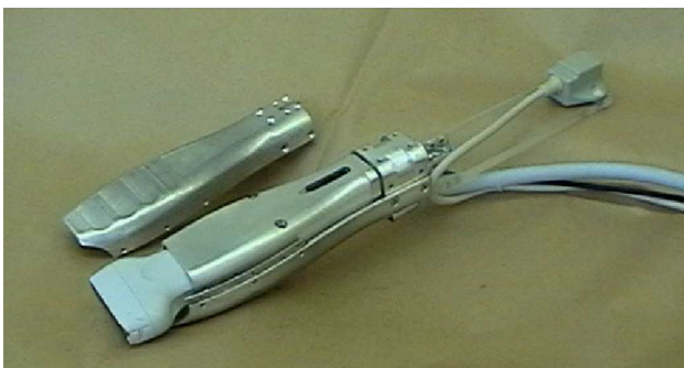
Fig. 3 Sensorized ultrasound probe used for data acquisition
