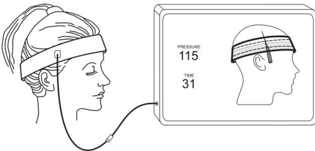
Figure 1. Personalized tourniquet system, with cuff applied to patient scalp and instrument displaying applied cuff pressure and inflation time.
